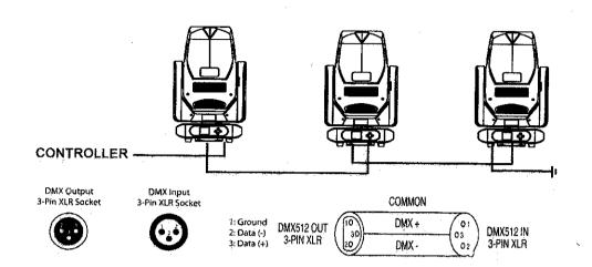
For installations where the DMX cable has to run a long distance or is in an electrically noisy environmentsuch as in a disco, it is recommended to use a DMX terminator. This helps in preventing corruption of the digital control singal by electrical noisy. The DMX terminator is simply an XLR plug with a 120 resistor connected between pins 2 and 3, which is then plugged into the output XLR Socket of the last fixture in the chain. Please see illustrations
